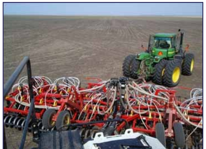
Source: Al Scholz – Bourgault air-drill seeding wheat on a single 1,800 acre field
